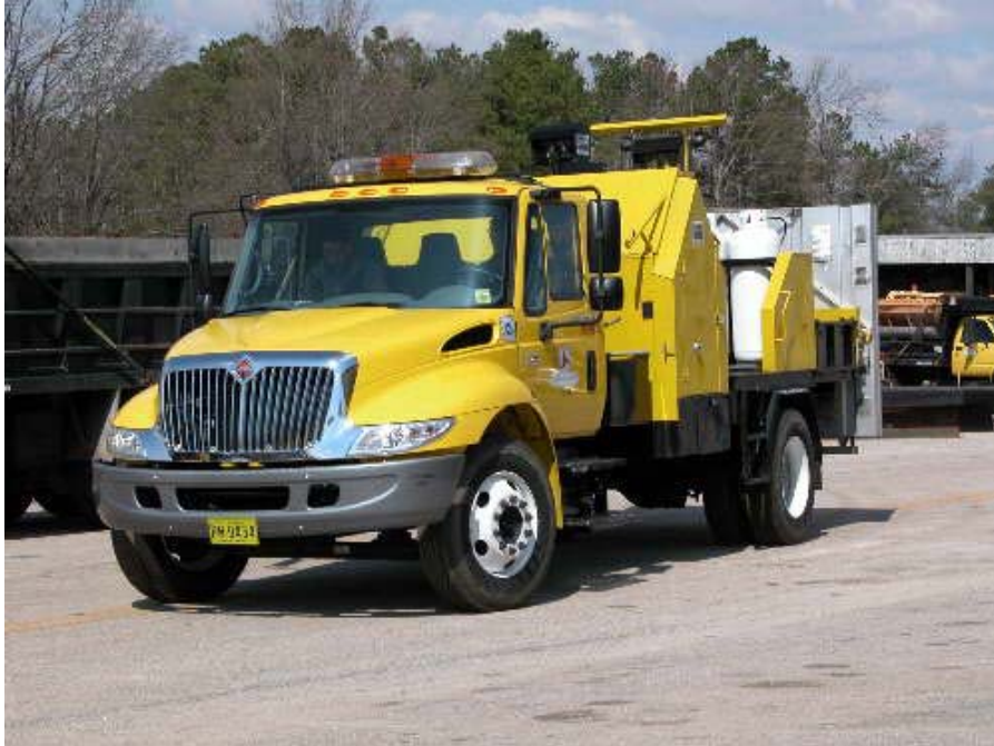
Figure 9. Instrumented NCDOT vehicle in motion as it leaves the maintenance yard after installation of the portable emissions measurement system..
