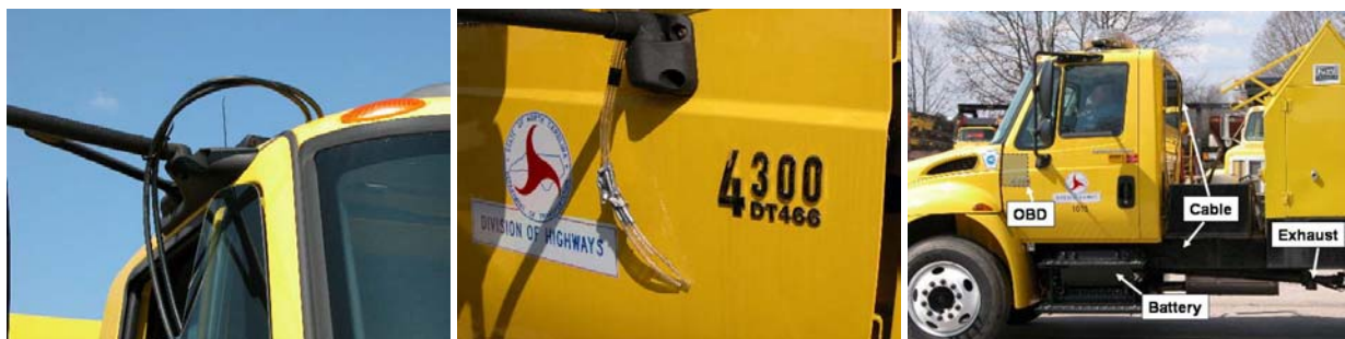
Figure 8. Installation of the portable emissions measurement system (PEMS) in a NCDOT heavy duty diesel vehicle: (a) routing sampling hoses through the window, secured with ties; (b) obtaining outdoor air for "zeroing"; (c) side-view of truck in motion, illustrating relative locations of the on-board diagnostic link (inside the vehicle), battery, exhaust, and cables/hoses.
