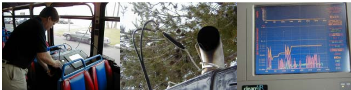
Figure 5. Example of a portable on-board emissions and fuel use measurement system installed in a heavy duty diesel transit bus: (a) the portable unit on a passenger seat; (b) the exhaust gas sampling probe; (c) the instrument display panel showing traces of emissions versus time.
