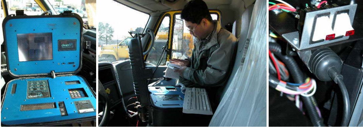
Figure 6. Installation of the portable emissions measurement system (PEMS) in a NCDOT heavy duty diesel vehicle: (a) the portable unit on a passenger seat; (b) entering vehicle data into the PEMS; (c) engine diagnostic link using a 9-pin Deutsch connector.
