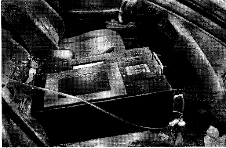
Figure 1. OEM-2100 installed in a 1998 Toyota Camry.
