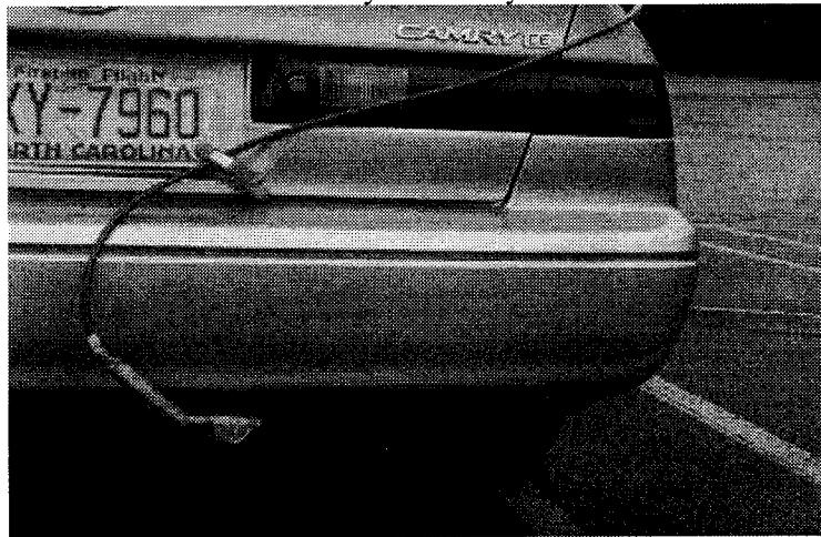
Figure 2. Sampling probe routed from vehicle tailpipe into vehicle, secured by clamps.
