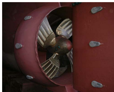
Figure 3.11 Nozzles Enclosing Propeller to Reduce Friction Losses
