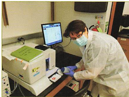
Figure 4. The Luminex LX-200 machine that was used to measure antibody responses in ORD's in-house multiplex salivary antibody assay.
