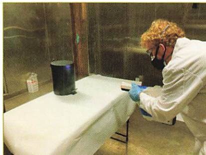
Figure 6. Testing of spraying a cylindrical object to investigate the ability of the electrostatic sprayer to have a claimed wrap around effect.
